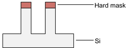
**3. Oxide deposition:** To isolate the fins from each other a oxide deposition with a high aspect ratio filling behavior is needed.
