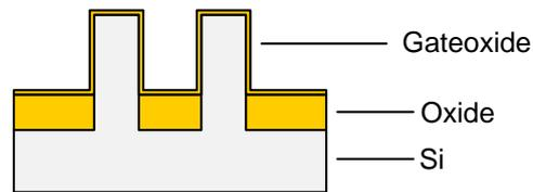
**7. Deposition of the gate:** Finally a highly  $n^+$ -doped poly silicon layer is deposited on top of the fins, thus up to three gates are wrapped around the channel: one on each side of the fin, and - depending on the thickness of the gate oxide on top - a third gate above.
