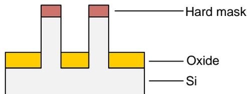
**6. Gate oxide:** On top of the fins the gate oxide is deposited via thermal oxidation to isolate the channel from the gate electrode. Since the fins are still connected underneath
