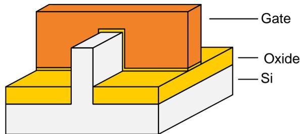
Fig. 1.1: FinFET in bulk process
