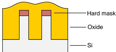
**4. Planarization:** The oxide is planarized by chemical mechanical polishing. The hard mask acts as a stop layer.
