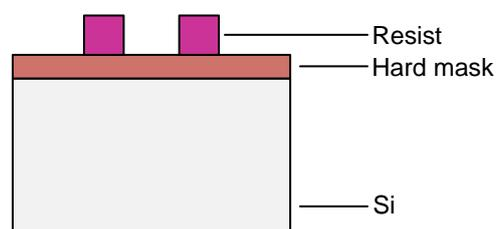
**2. Fin etch:** The fins are formed in a highly anisotropic etch process. Since there is no stop layer on a bulk wafer as it is in SOI, the etch process has to be time based. In a
