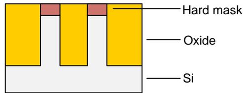
**5. Recess etch:** Another etch process is needed to recess the oxide film to form a lateral isolation of the fins.
